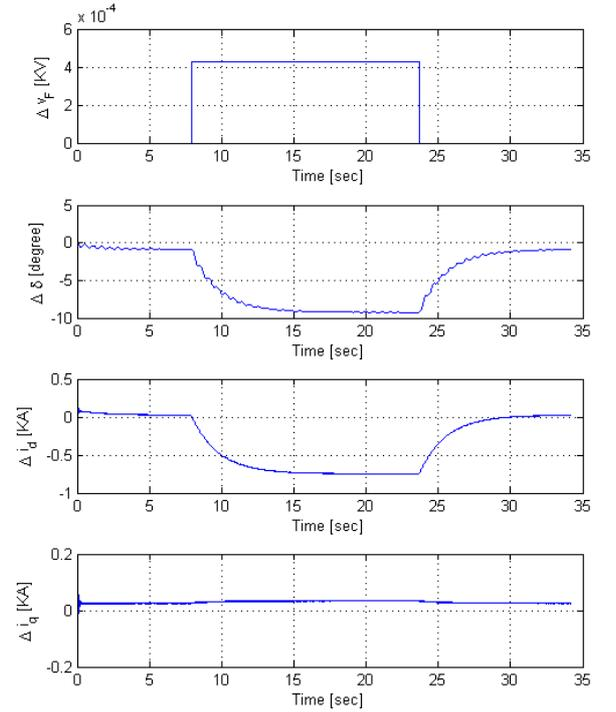
Fig. 4. Response to the exciter voltage step change of the controlled generator ( $\Delta$  means the deviation from the steady-state value)
