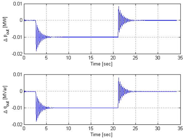
Fig. 5. Changing the effective power of the generator
