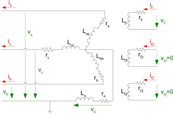
Fig. 2. The simplified schema of the synchronous machine
