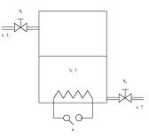
Construct the model of the coffee machine if we can measure the water level, the water temperature and the status of the valves and the switch.
