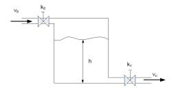
Construct the model of the tank for diagnostic purposes if we can measure the water level and the status of the valves.
