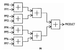
Figure 3.15. Multiplication by Direct Methods: Linear and Tree.
