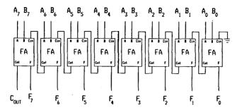
Figure 33. A Word Adder Composed of Full Adders.
