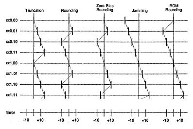
Figure 3.27. Errors in Handling Extra Bits.
