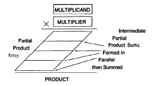
Figure 3.19. Partial Product Reduction by Sectioning.
