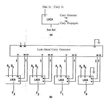
Figure 35. Look-Ahcad Carry Adder (LACA) and its Connection in an Adder Circuit.
