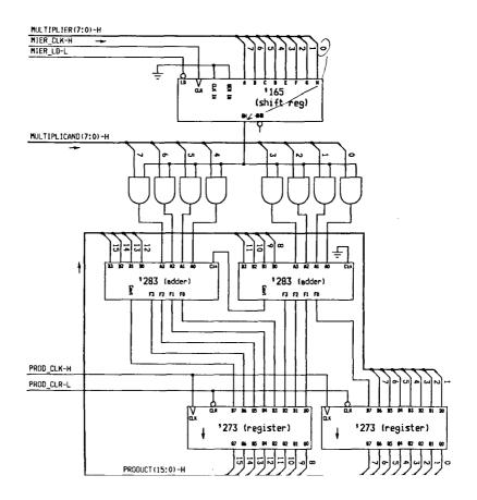
Figure 3.9. Data Path Logic Diagram for Simple Multiplier.
