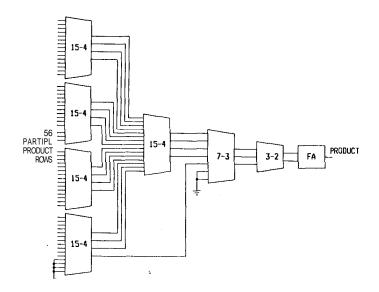
Figure 3.18. 56-Bit Multiplication Using Row Reduction.
