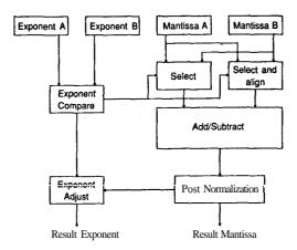
Figure 3.25. Block Diagram for Floating Point Addition.
