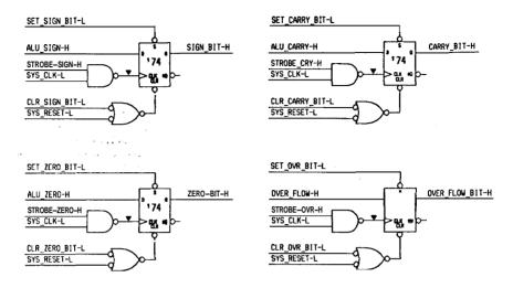
Figure 3.8. Arithmetic Bit Formation for a Status Register.
