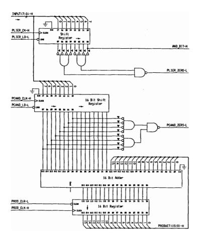
Figure 3.12. Data Path for Multiplier of Example 3.3
