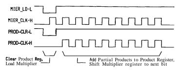
Figure 3.10. Timing of Control Signals for Simple Multiplier.
