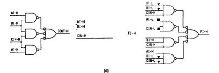
Figure 3.2. Design of a Full Adder (FA).
