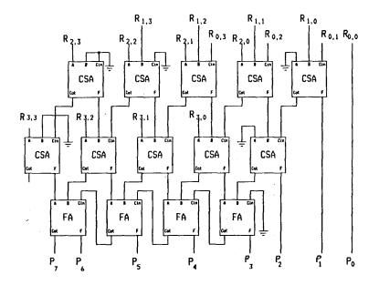
Figure 3.17. Partial Product Addition with Carry Save Adders.
