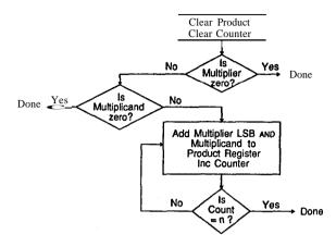
Figure 3.11. Flow Diagram for Data Dependent Multiply Algorithm.
