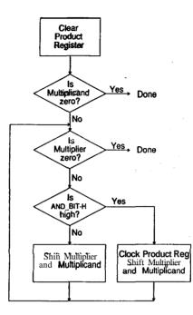
Figure 3.13. Flow Diagram for Multiplier of Example 3.3.
