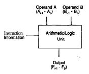
Figure 3.1. Connections for an Arithmetic/Logic Unit.
