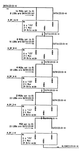
Figure 3.26. Logic for Alignment Shift Network.
