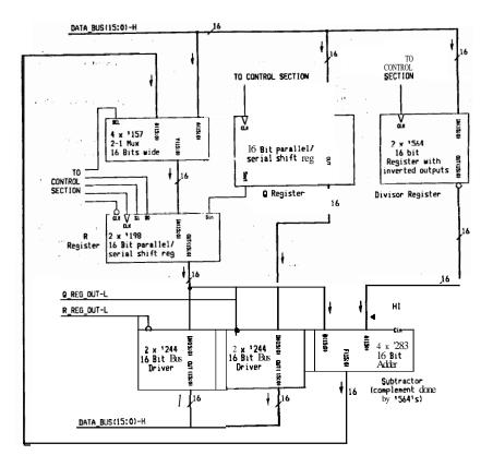
Figure 3.23. Logic for Divide Operation.
