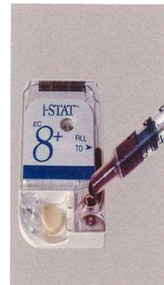
Collect just 2-3 drops of fresh whole blood and fill cartridge.
