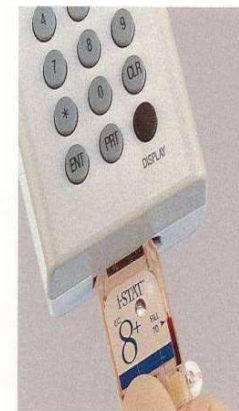
Insert cartridge into the portable, battery-powered analyzer.
