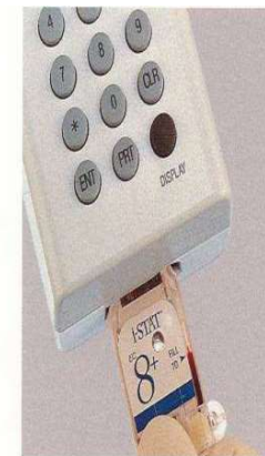
Insert cartridge into the portable, battery-powered analyzer.
