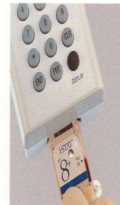
Insert cartridge into the portable, battery-powered analyzer.
